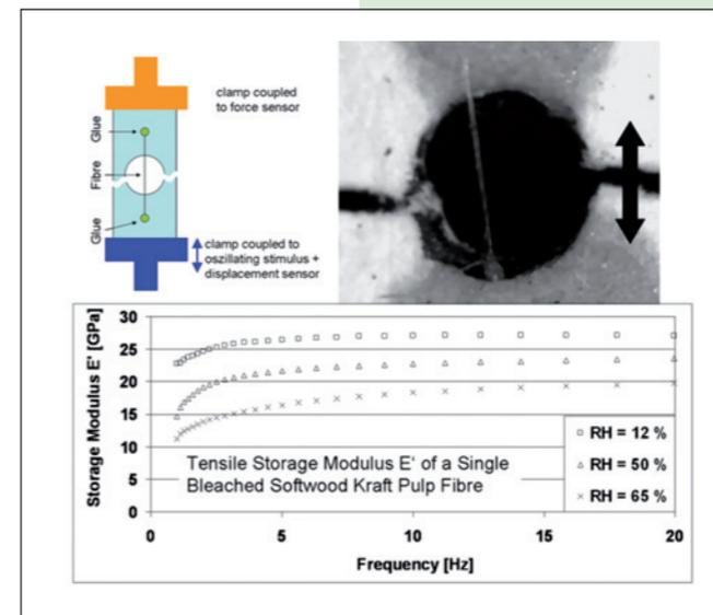
Measuring principle of Dynamic Mechanical Analysis and first results of single fibre characterization
