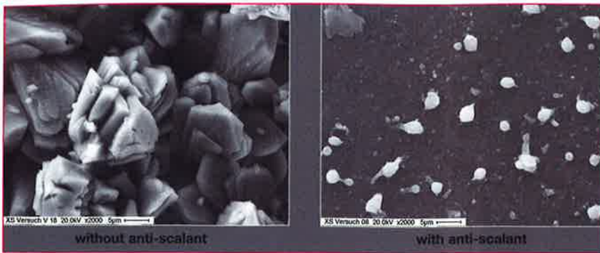
Fig. 5: Calcium carbonate deposits on a membrane: The effect of antiscalants is clearly visible in the SEM image (lecture by T. Richter, BK Giulini GmbH)
