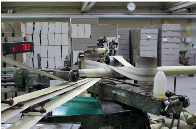
**Fig. 6:** Demonstration scale conversion of papers with 25 % share of hop residue pulp into paper cores
