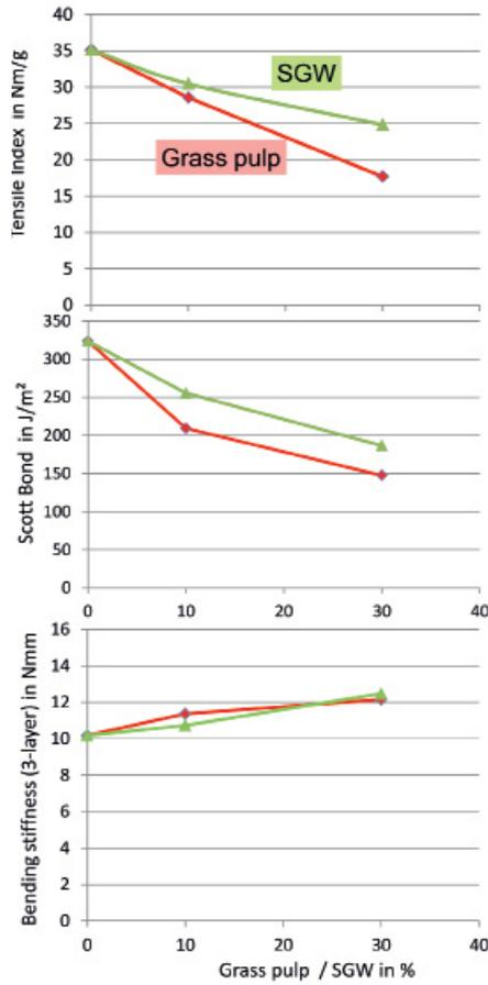
**Fig. 7:** Comparison of the effect of mechanically prepared grass pulp and stone-ground wood (SGW) market pulp on major board properties when substituted for recycled fibre pulp. Bending stiffness for a three-layer board was calculated based on a laminate-theory modul
